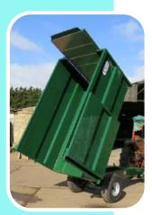
• To empty the trailer a single piece rear door is hinged sideways and folds back onto the side of the trailer, this prevents the door sticking into the muck heap when tipped.
