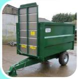
Designed as a front loading trailer, the front headboard folds down over the drawbar, the weight is taken by two tension springs so raising and lowering the ramp requires little effort.
